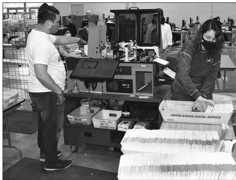
This machine and seven others like it were used for automated signature verification, comparing voter signatures to DMV signatures and others on file in the system. Ballots with signatures are stacked up in the tray at the far right of the machine, similar to the output tray of a photocopier. But see that little gray box at lower right with four or five ballots in there on an angle? If the ballot has no signature, a little trap door opens and the envelope drops down in that area for manual processing of signature comparison.
